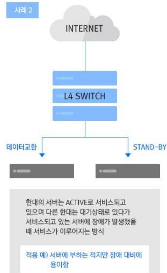
The server is being serviced as active, the other is in standby, and the service is performed when the server being serviced fails.
